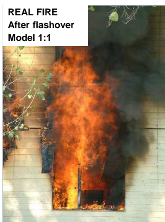
Figure 6 Flame and smoke propagation during façade fire Comparison of real fire (LEFT) and CFD modeling (RIGHT)
