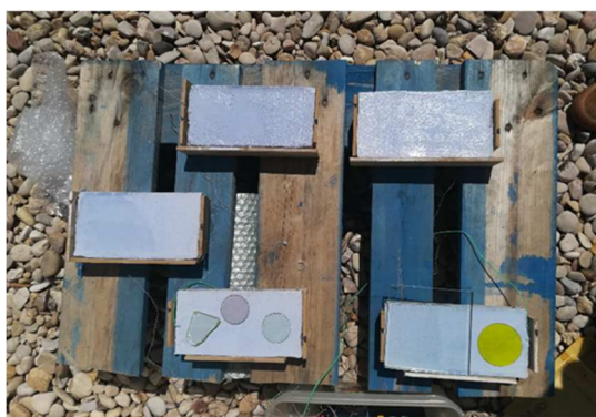
Figure 1.: Location of thermochromic mortar coated tiles during the test (left) and transmittance spectra of the glass protections (right).
