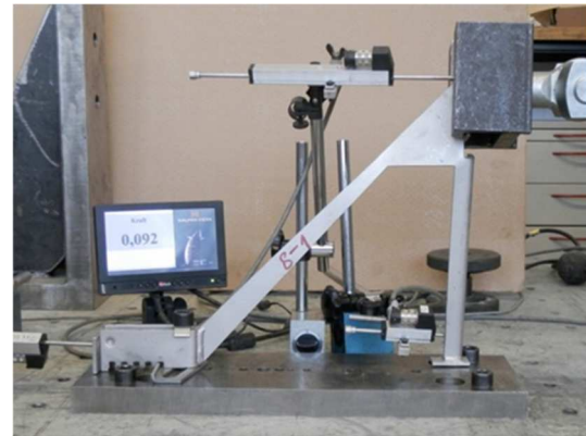
Figure 13: masonry bracket after test
