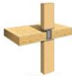
CLT floor slab with glulam column and steel connector
