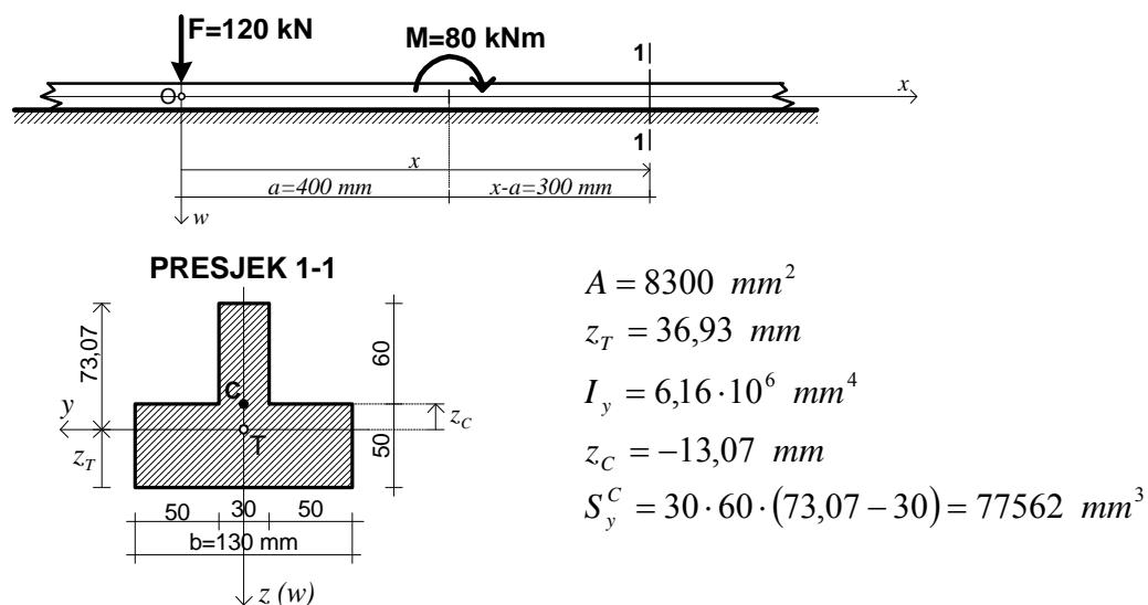
Koeficijent podloge:  $k = k_1 \cdot b = 8000 \cdot 0,13 = 1040 \text{ MN/m}^2 = 1040 \text{ MPa (N/mm}^2)$
