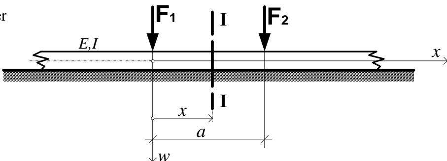
$$w = \frac{F_1}{8EI\alpha^3} \cdot e^{-\alpha x} (\sin \alpha x + \cos \alpha x) + \frac{F_2}{8EI\alpha^3} \cdot e^{-\alpha(a-x)} [\sin \alpha(a-x) + \cos \alpha(a-x)]$$
