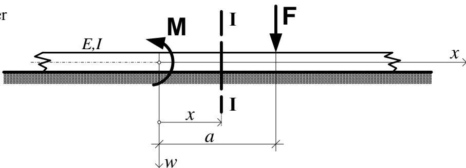
$$w = -\frac{M}{4EI\alpha^2} \cdot e^{-\alpha x} \sin \alpha x + \frac{F}{8EI\alpha^3} \cdot e^{-\alpha(a-x)} [\cos \alpha(a-x) + \sin \alpha(a-x)]$$
