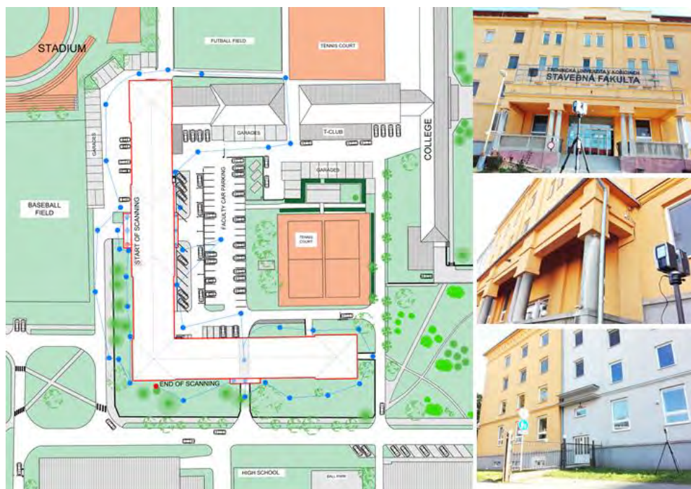
Figure 24. Technological process of terrestrial laser scanning/focused on the facade from the building (source: authors)
