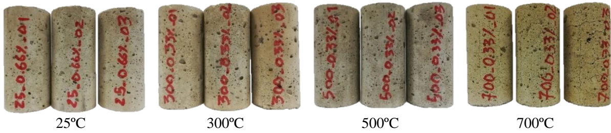
Figure 3: Visual appearance of the specimens after high temperature exposure.
