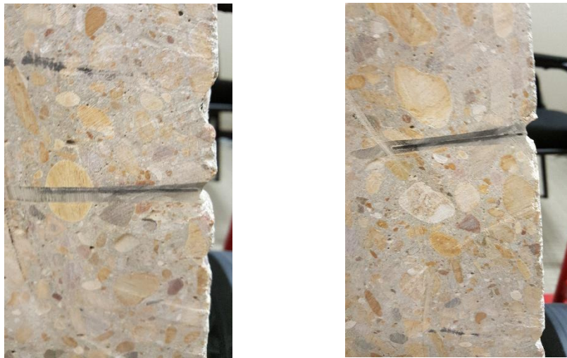
Figure 8: Saw cut of test slab showing the FRP strip well positioned with respect to the slot and excellent bonding with the base concrete
