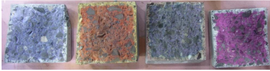
Figure 3: Colour change on a concrete sample determined with different indicators (from left to right: 0.1 % thymolphthalein, 0.5% curcumin, Rainbow Indicator, 1% phenolphthalein)
