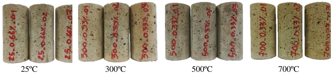
Figure 3. A change in the colour of the specimens is observed with the increase of the temperature exposure. The presence of relatively large cracks is noticed for specimens exposed to 700°C. The specific weight of the specimens was measured before and after the thermal treatment, being 16.80, 15.73, 15.51 and 15.13 kN/m 3 for 25, 300, 500 and 700°C, respectively.
