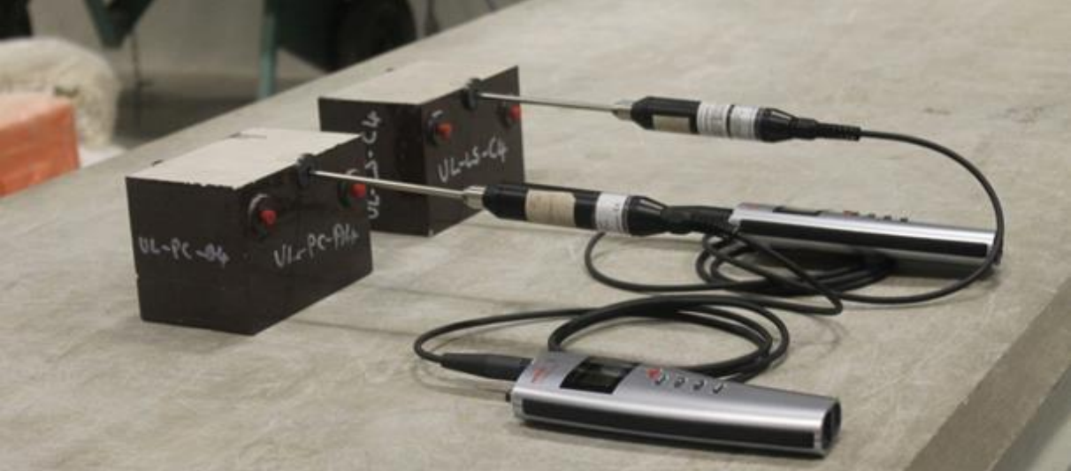
Figure 2: Experimental program for RH measurement
