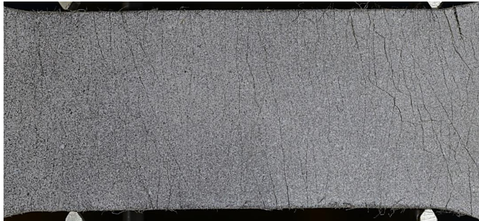
Figure 2: Close-up of the cracked surface of the ECC dogbone specimen after tensile testing. The longitudinal distance between pins is 110 mm and the transverse is 50 mm.
