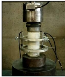
Figure 2: Set-up of static E-modulus
