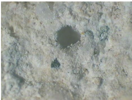
Figure 6a: Secondary crystallization in pores
