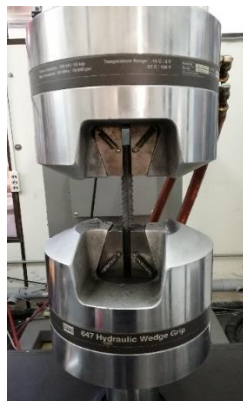
Figure 3: (Left) Experimental fatigue test (free length 96 mm). (Right) Strain waveforms received as input
