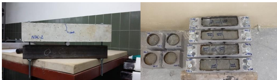
Figure 1: Experiment setup for salt scaling
