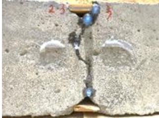
Figure 7: Release of repair agent outside the specimen
