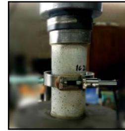
Figure 3: Set-up of Poisson's ratio
