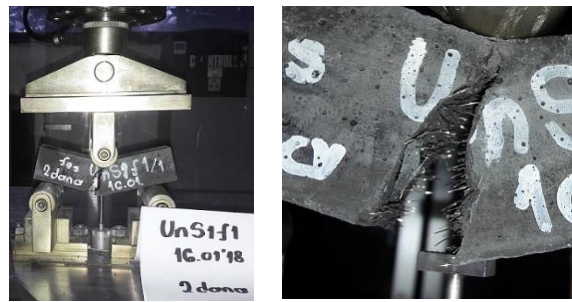
Figure 1. Testing tensile strength beams and its cross-section
