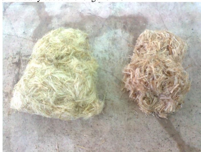
Figure 1: Spanish broom (left) and hemp (right) fibers
