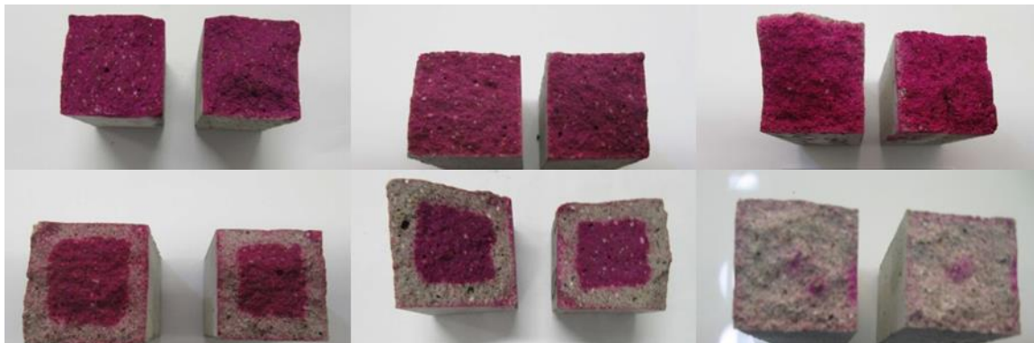
Figure 2: Carbonation depth of mortars after 28 day curing in air (up) and 56 days of exposure to accelerated carbonation (below): left : reference mixture, middle : 20% of K4 ; right : 20% of K5.
