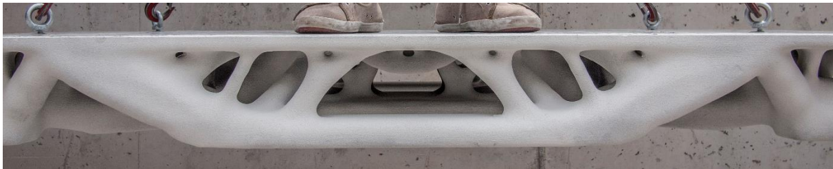
Figure 1: Stay-in place formwork for a concrete slab 3D printed with organic binder. High performance fiber reinforced concrete is poured inside. (Image: Chair of digital building technologies)
