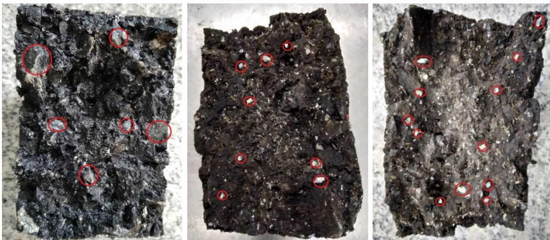
(a) Reference CBEM (b) CBEM with superplasticizer (c) CBEM with superplasticizer and JFC Figure 8 Fracture face of hardened CBEM (3.9% of water content)
