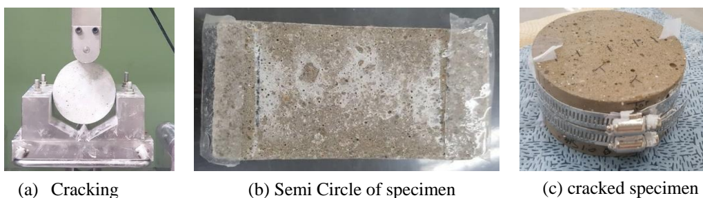
Figure 1: Preparation of cracked specimen
