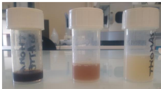
Figure 5 - Pore solutions extracted from AAS- \text{Na}_2\text{SiO}_3 samples. Left is after 3 days. Centre is after 7 days. Right is after 28 days.
