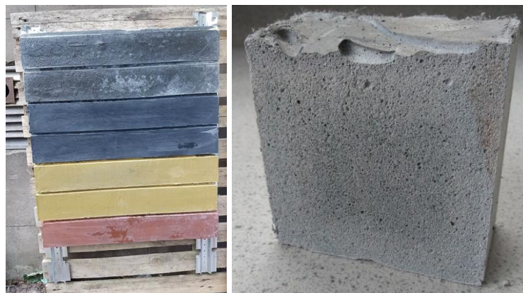
Figure 3. Rainscreen façade elements cast with pigmented geopolymer concretes and a lightweight geopolymer foamed concrete sample made using a pre-formed foam technique, manufactured in Queen’s University Belfast
