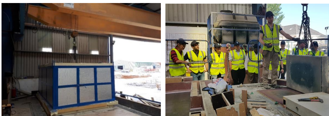
Figure 1. Curing chamber in use during manufacturing and specimens being demoulded during partner visits – May 2018
