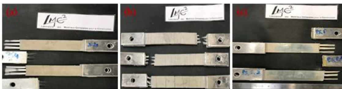
Figure 5: 3Y composites failure modes (a) D, (b) PIW.K3 and (c) PID.SAC
