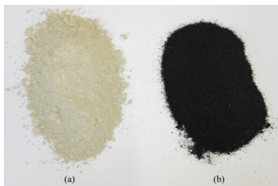
Figure 1. Materials used as a filler replacement in experimental work: (a) wood biomass ash (WBA); (b) tire powder (TP)
