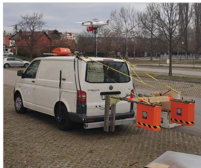
— GPR System used for pavement thickness measurement and road condition assessment
