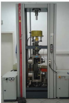
— Universal Testing Machine for testing of various geosynthetic materials
