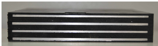
Fig. 1: Cross section of a laminated elastomeric bearing 200x300x41 mm
