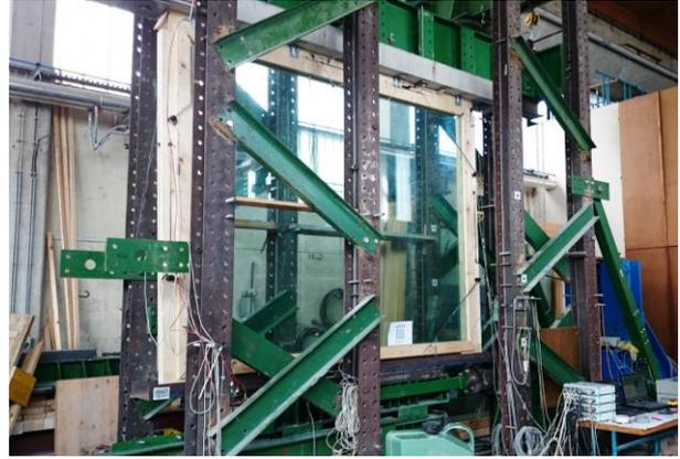
Figure 1: Hybrid system made of timber and structural glass [1–7] as tested in the laboratory of University of Ljubljana
