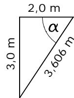
$$\begin{aligned}\sum M_A &= 0 \\ S_1 \cdot 4,0 - S_2 \sin \alpha \cdot 2,0 &= 0 \\ S_1 &= \frac{1}{2} S_2 \sin \alpha\end{aligned}\quad (1)$$
