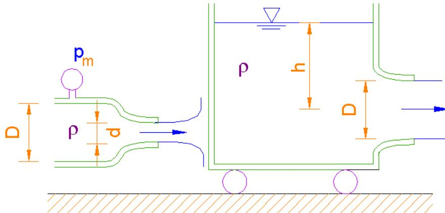
$$\rho v_d^2 \cdot \frac{d^2 \pi}{4} = \rho v_{D \text{ kolica}}^2 \frac{D^2 \pi}{4} \quad / \cdot \frac{4}{\rho \pi} \quad (\text{ravnoteža sile koje djeluju na kolica})$$
