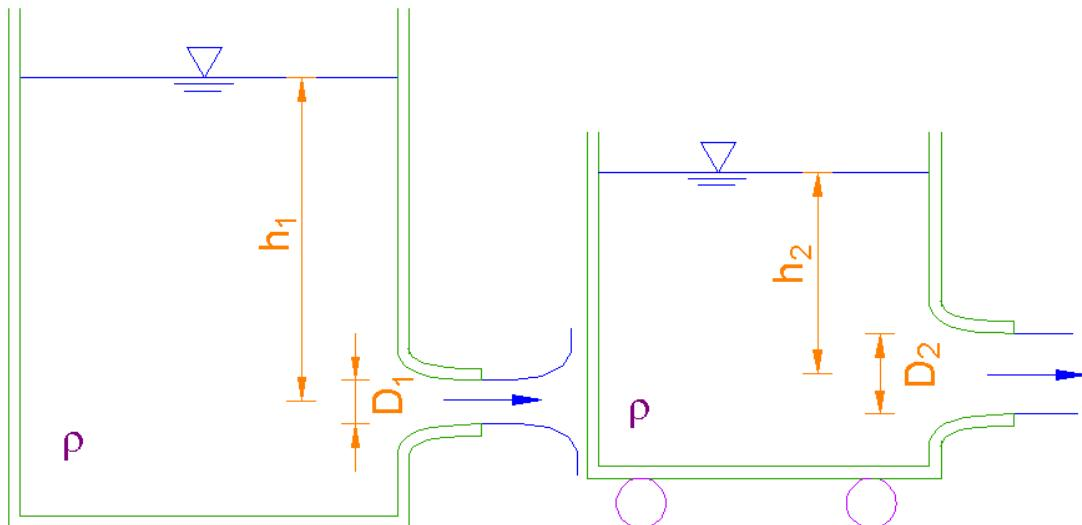
$$\rho Q_2 v_2 = \rho Q_1 v_1$$
