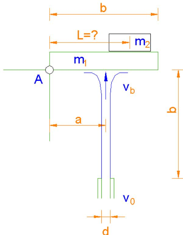
$$Q = v_0 \cdot \frac{d^2 \pi}{4} = 10 \cdot \frac{0,25^2 \pi}{4} = 0,491 \text{ m}^3 / \text{s}$$
