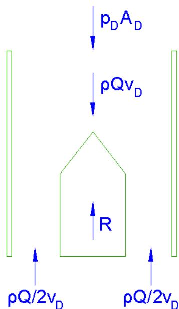
$$v_D = \frac{Q}{A_D} = \frac{Q}{D^2} = \frac{2}{1^2} = 2 \text{ m/s} \quad \frac{v_D^2}{2g} = 0,20 \text{ m}$$
