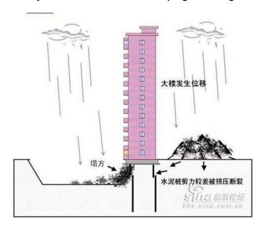
The building began to tilt. Then it began to shift, and the "hollow" concrete pilings were snapped due to the uneven lateral pressures.
