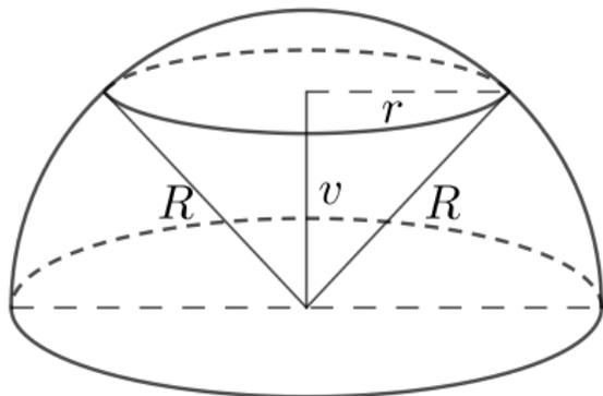
$$\begin{aligned}R^2 &= v^2 + r^2 \\r^2 &= R^2 - v^2\end{aligned}$$
