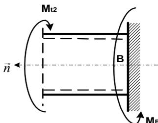
$$\begin{aligned} \sum M_x = 0 &\Rightarrow M_{t2} - M_B = 0 \\ &\Rightarrow M_{t2} = M_B \end{aligned}$$
