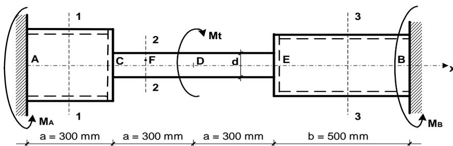
$$\begin{aligned} \sum M_x &= 0 \\ M_A - M_t + M_B &= 0 \\ M_A + M_B &= M_t \quad (1) \end{aligned}$$
