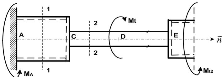
$$\begin{aligned} \sum M_x = 0 &\Rightarrow M_A - M_t + M_{t2} = 0 \\ &\Rightarrow M_{t2} = M_t - M_A \\ \text{iz uvjeta ravnoteže } M_t - M_A &= M_B \\ &\Rightarrow M_{t2} = M_B \end{aligned}$$
