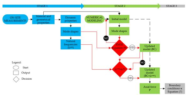
Figure 4. Methodology for boundary conditions determination.
