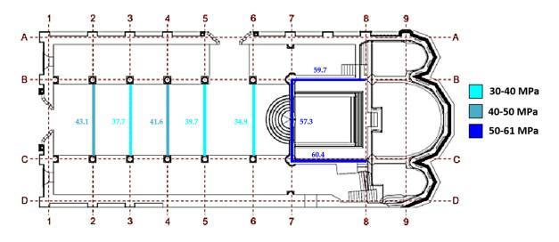
Figure 14. Stress levels measured on the tie rods in the Cathedral of St. James in Šibenik at level R4.
