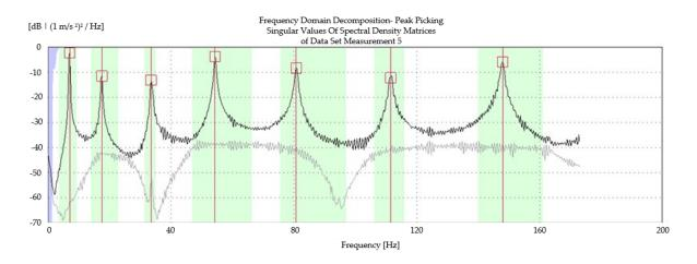
**Figure 10.** Characteristic record of frequency domain decomposition (FDD) for the determination of natural frequencies on reference iron tie rod 6B–C.
