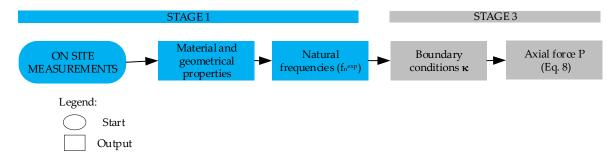
Figure 5. Methodology for axial load identification.
