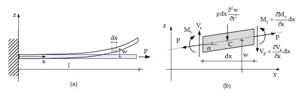
**Figure 3.** (**a**) Beam under lateral vibration and axial loading and (**b**) differential segment of beam representing the positive orientation of bending moments, shear forces, and axial and inertial forces of mass.
