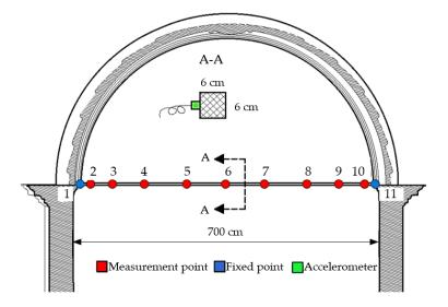
Figure 8. Reference tie rod (6B–C, R4) with measuring points and dimensions.
