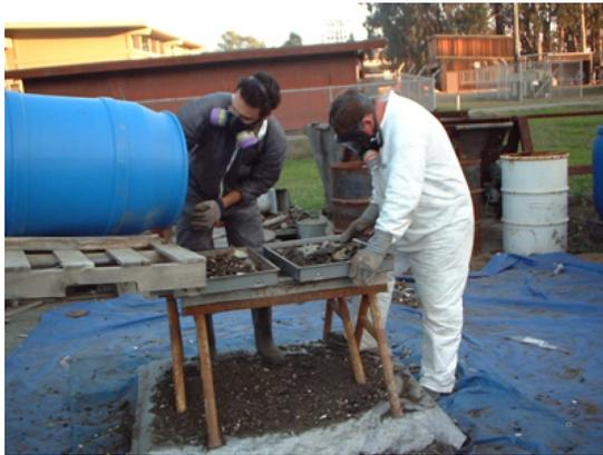
Fig. 6. Processing of the waste through the 20-mm sieve
