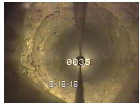
**Fig. 4.** View of the layered structure of the OII waste at a depth of 10.7 m
