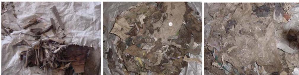
**Fig. 10.** View of the primary waste constituents of the >20-mm fraction for Tri-Cities waste: wood, paper, and plastic (from left to right)
