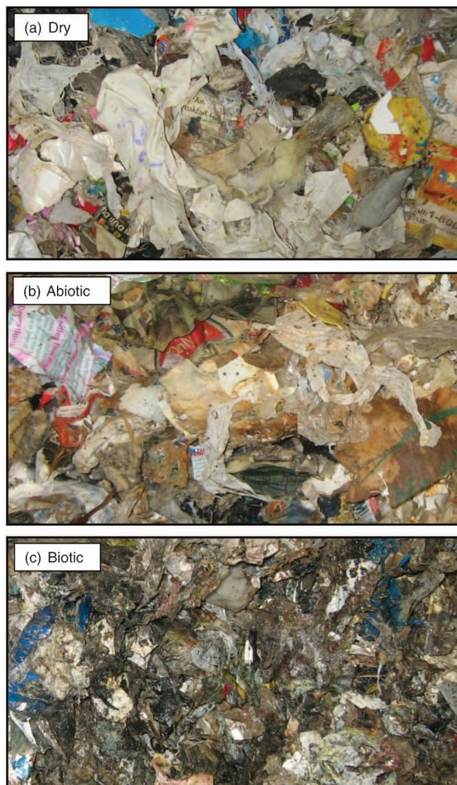
**Fig. 8.** (Color) Municipal solid waste recovered from (a) dry; (b) abiotic; and (c) biotic test cells at the end of reactor operation
