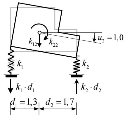
$$\begin{aligned} \sum F_z &= 0 \\ k_{12} + k_1 \cdot d_1 - k_2 \cdot d_2 &= 0 \\ k_{12} &= k_2 \cdot d_2 - k_1 \cdot d_1 = -9000 \text{ kN} \end{aligned}$$
