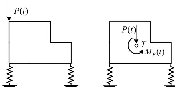
$$\{p(t)\} = \begin{Bmatrix} p_1(t) \\ p_2(t) \end{Bmatrix} = \begin{Bmatrix} P(t) \\ M_p(t) \end{Bmatrix} = \begin{Bmatrix} 50 \sin(10t) \\ -50 \sin(10t) \cdot 1,3 \end{Bmatrix} = \begin{Bmatrix} 50 \sin(10t) \\ -65 \sin(10t) \end{Bmatrix}$$
