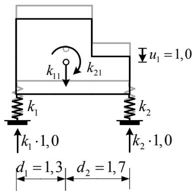
$$\begin{aligned} \sum F_z &= 0 \\ k_{11} - k_1 - k_2 &= 0 \\ k_{11} &= k_1 + k_2 = 30000 \text{ kN/m} \end{aligned}$$
