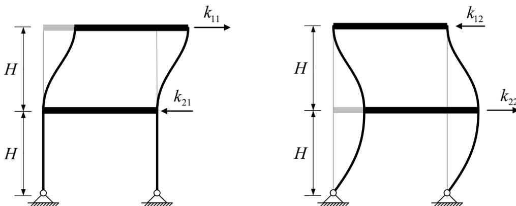
$$k_{11} = 2 \frac{12EI}{H^3} = 56888,9 \text{ kN/m} \qquad k_{21} = -k_{11} = -2 \frac{12EI}{H^3} = -56888,9 \text{ kN/m}$$
