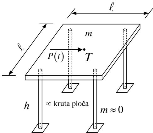
$$h = 6 \text{ m}, \ell = 8 \text{ m}, t_p = 30 \text{ cm} \quad k = 523,6 \text{ kN/m}$$
