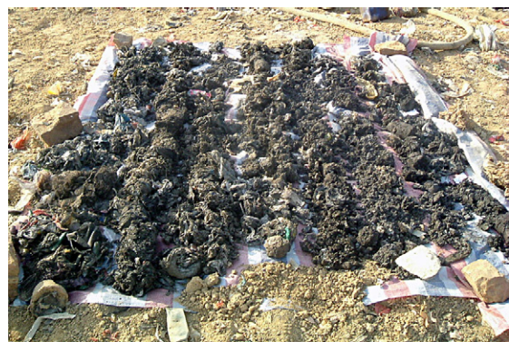
Fig. 3. Disturbed MSW samples taken at different depths (i.e., embedment depth increases from left to right).
