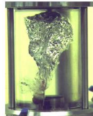
c) Aluminium foil surrounding inflated balloon for diffusion reduction
