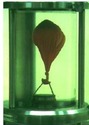
b) Due to water pressure, the volume of the balloon decreases and pressure equilibrium is reached. The membrane is completely unloaded.
