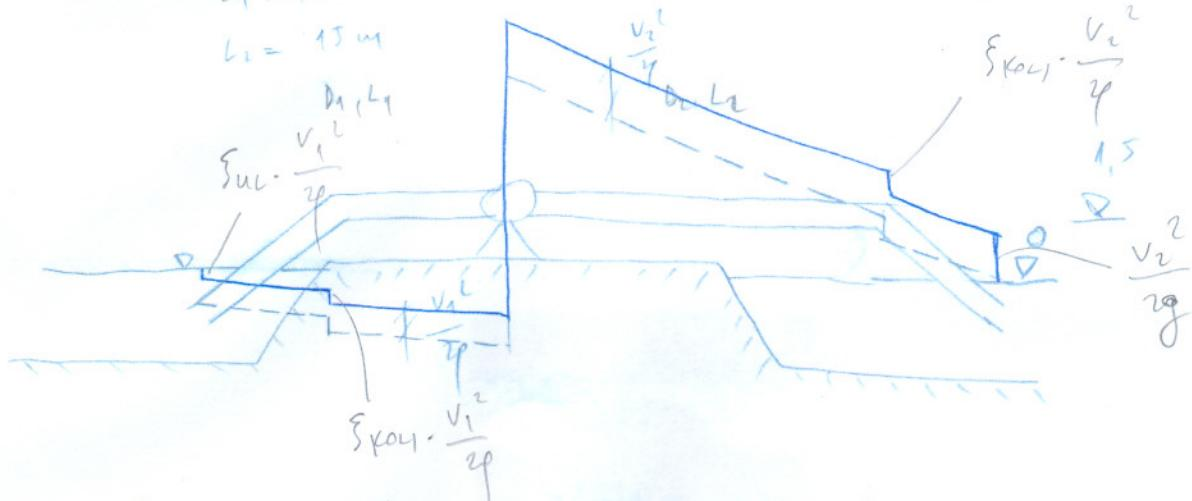
$$v_1 = \frac{Q \cdot h}{D_1^2 \pi} = \frac{0,015 \cdot 4}{0,1^2 \cdot \pi} = 1,91 \text{ m/s} ; R_{c1} = \frac{v_1 \cdot D_1}{\nu} = \frac{1,91 \cdot 0,1}{1,01 \cdot 10^{-6}} = 1,9 \cdot 10^5$$
