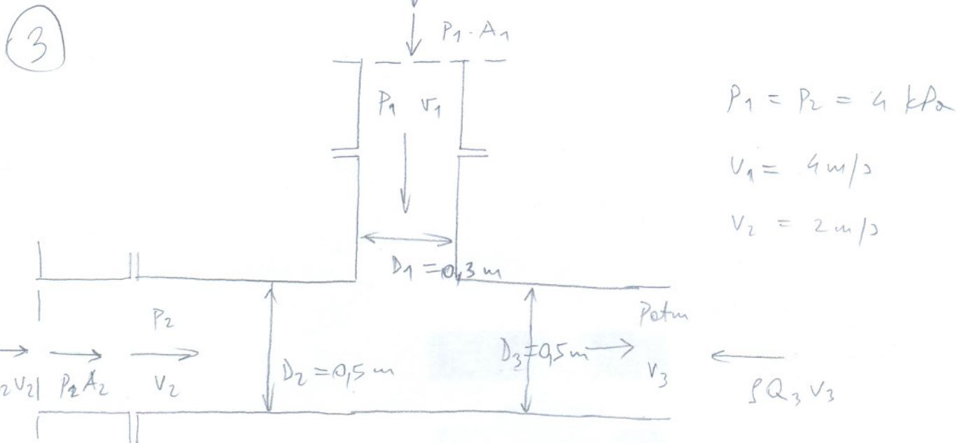
$$Q_1 = A_1 \cdot v_1 = \frac{D_1^2 \pi}{4} \cdot v_1 = \frac{0.3^2 \pi}{4} \cdot 4 = 0.283 \text{ m}^3/\text{s}$$
