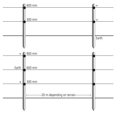
Low-level electric fences can be be semi permanent as here or temporary. Above: Energised 2 wire fence with 3 wire fence below.
