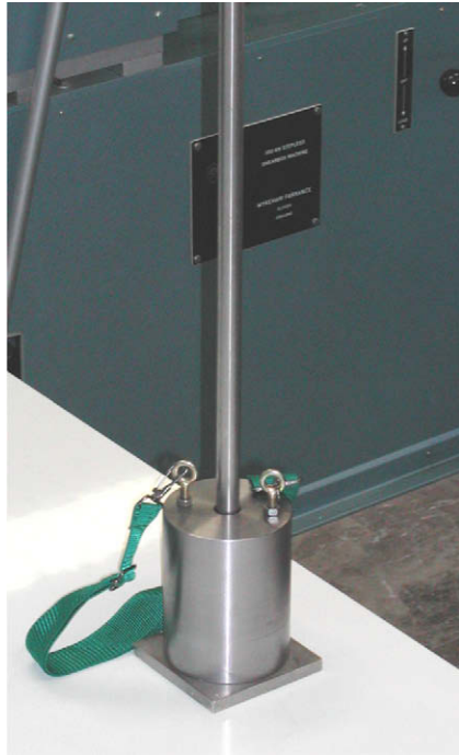
Fig. 4. Drop weight used for the MSW specimen preparation.
