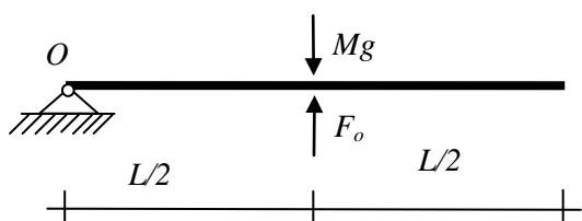
$$\begin{aligned} \sum M_O &= 0 \\ Mg \frac{L}{2} - F_o \frac{L}{2} &= 0 \quad \Rightarrow F_o = Mg = k \cdot \delta_{o1}, \quad \delta_{o1} = \frac{x_{st1}}{2} \\ \delta_{o1} = \frac{Mg}{k} &\Rightarrow x_{st1} = \frac{2Mg}{k} \end{aligned}$$
