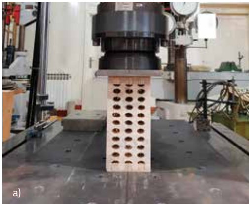
Innovative glued-laminated wooden elements: a) elliptical hollows; b) circular perforations
