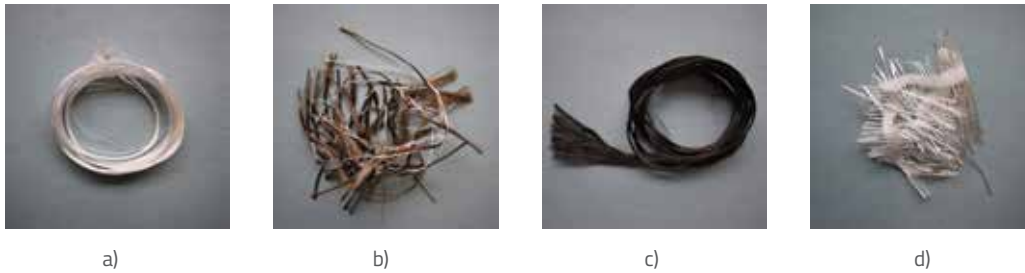
Waste fibres from the production of high-performance textiles for construction industry: a) glass fibres – roving end, b) basalt fibres – scrap from production, c) carbon fibres – roving end, d) glass fibres – scrap from production.
