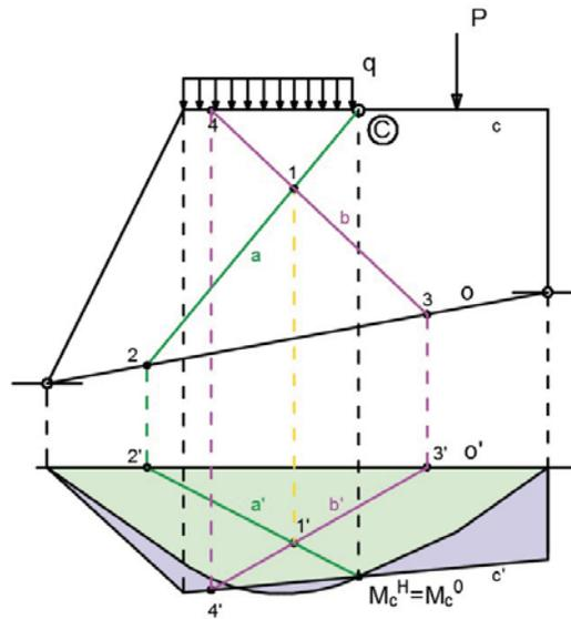
Figure 4: Construction of the affine image of the frame
