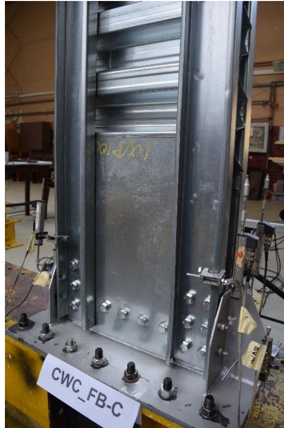
Cyclic bending test on laser welded column
