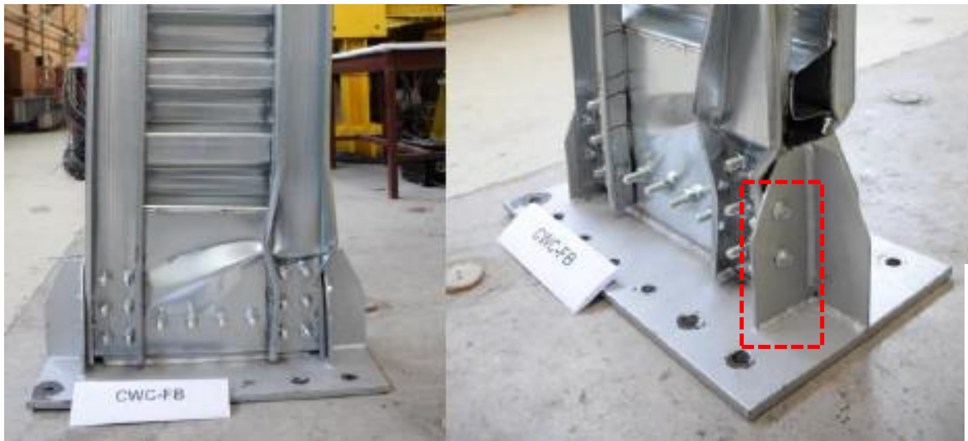
After-test image of the column with bolted flanges (CWC-FB) subjected to monotonic displacement
