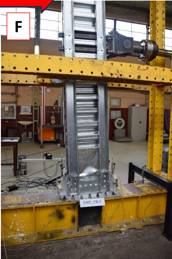
Cyclic bending test on laser welded column
