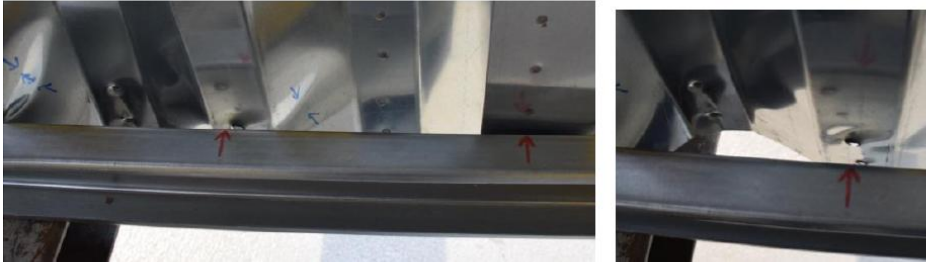
Spot welding failure between the web and the flange
