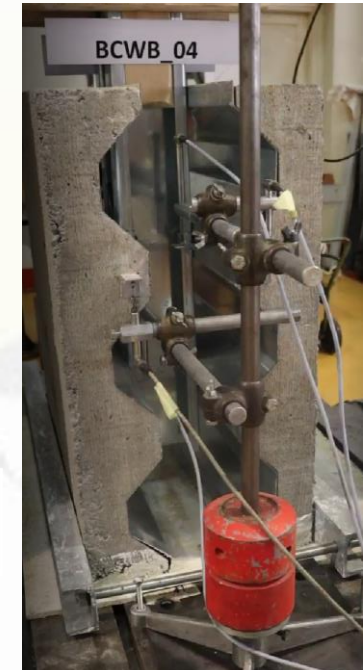
b) Demountable headed shear studs connectors
