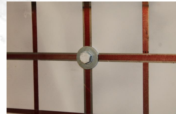
Infill steel plate hole bearing failure (CPSW)
