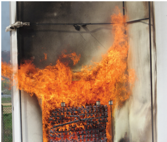
Fire resistance testing of facades
