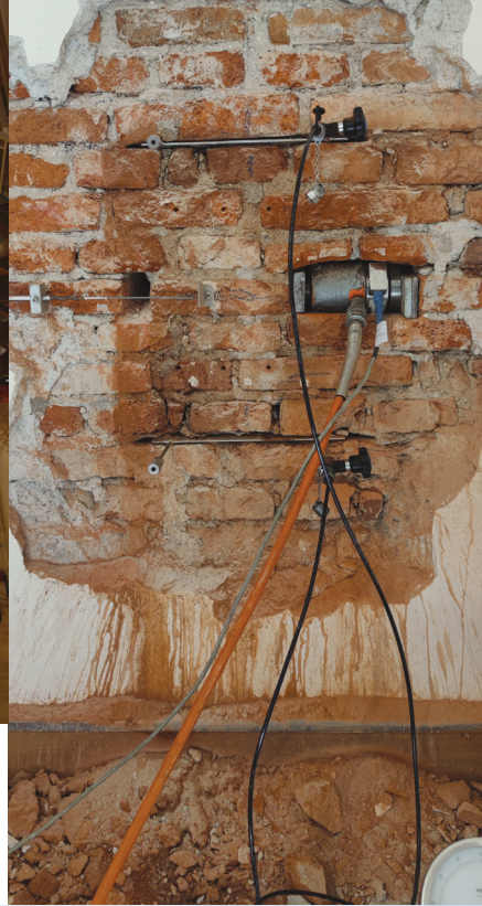
— Masonry shear strength testing with flat jacks
