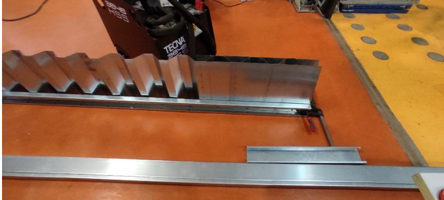
Spot-welding of built-up CFS
