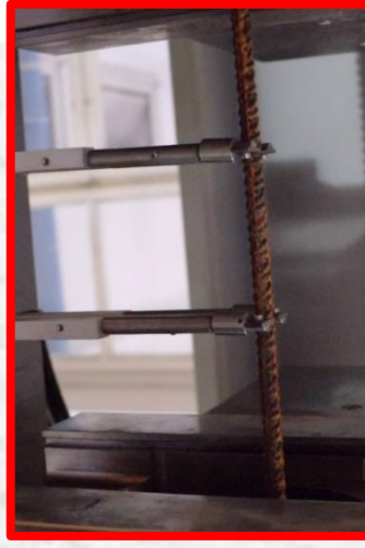
Reinforcement: bars 8 mm and mesh 10 mm, B500, 10 specimens
