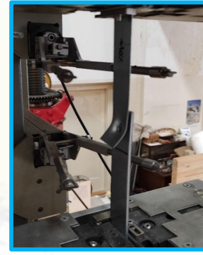
Spot welds: different combinations of steel sheet thicknesses, 558 specimens
