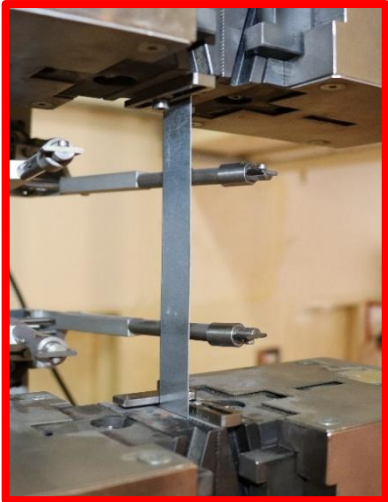
Steel sheets: 0,8 mm, 1,0 mm, 1,25 mm, 1,5 mm, 2,0 mm, 2,5 mm and 3,0 mm, steel grades DX51 and GD 350 for 3,0 mm only, 135 specimens
