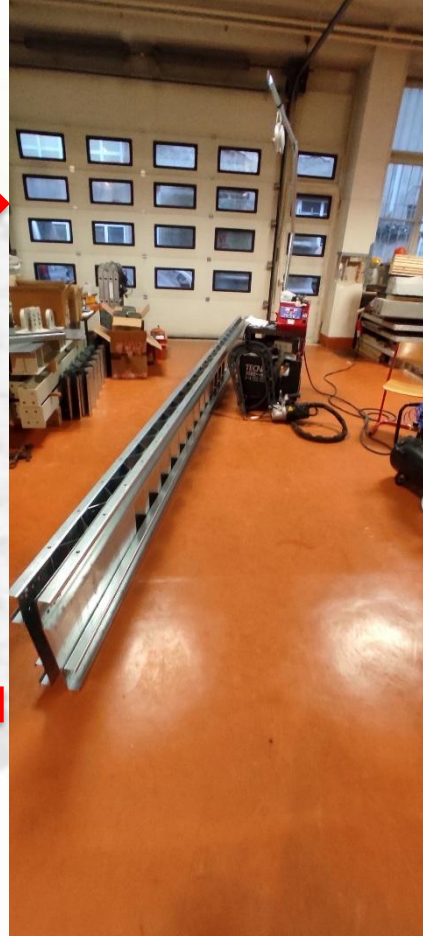
Fabricated steel specimens
