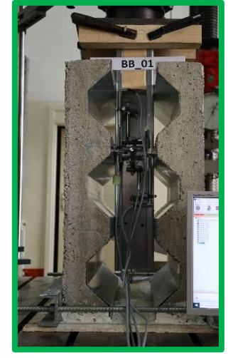
Shear connections: different types (with concrete dowels (LC and NC) and demountable types with and without additional corrugated web (NC only)), 30 specimens
