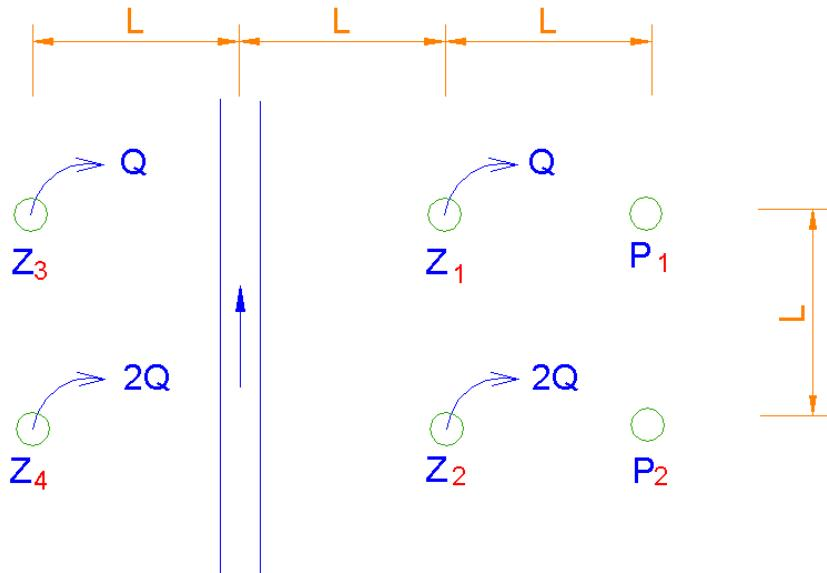
$$s_{P1} = \frac{Q}{2\pi k M} \ln \frac{R}{L} + \frac{2Q}{2\pi k M} \ln \frac{R}{L\sqrt{2}} = 0,828 \text{ m}$$
