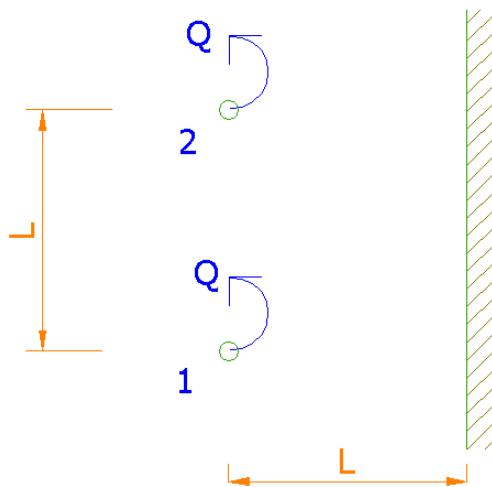
$$s_1 = \frac{Q}{2\pi k M} \ln \frac{R}{r_0} + \frac{Q}{2\pi k M} \ln \frac{R}{L} + \frac{Q}{2\pi k M} \ln \frac{R}{\sqrt{L^2 + (2L)^2}} + \frac{Q}{2\pi k M} \ln \frac{R}{2L}$$
