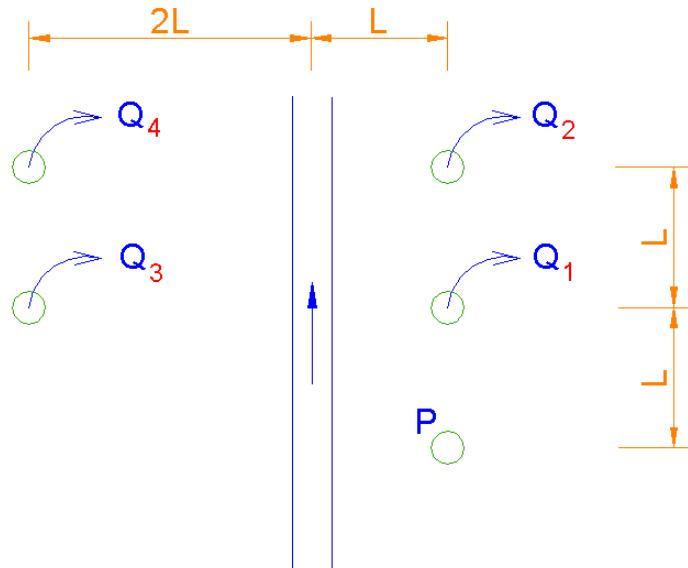
$$\Delta\Phi = \frac{Q_1}{2\pi} \ln \frac{R}{50} + \frac{Q_2}{2\pi} \ln \frac{R}{100} - \frac{Q_1}{2\pi} \ln \frac{R}{\sqrt{100^2 + 50^2}} - \frac{Q_2}{2\pi} \ln \frac{R}{\sqrt{100^2 + 100^2}}$$
