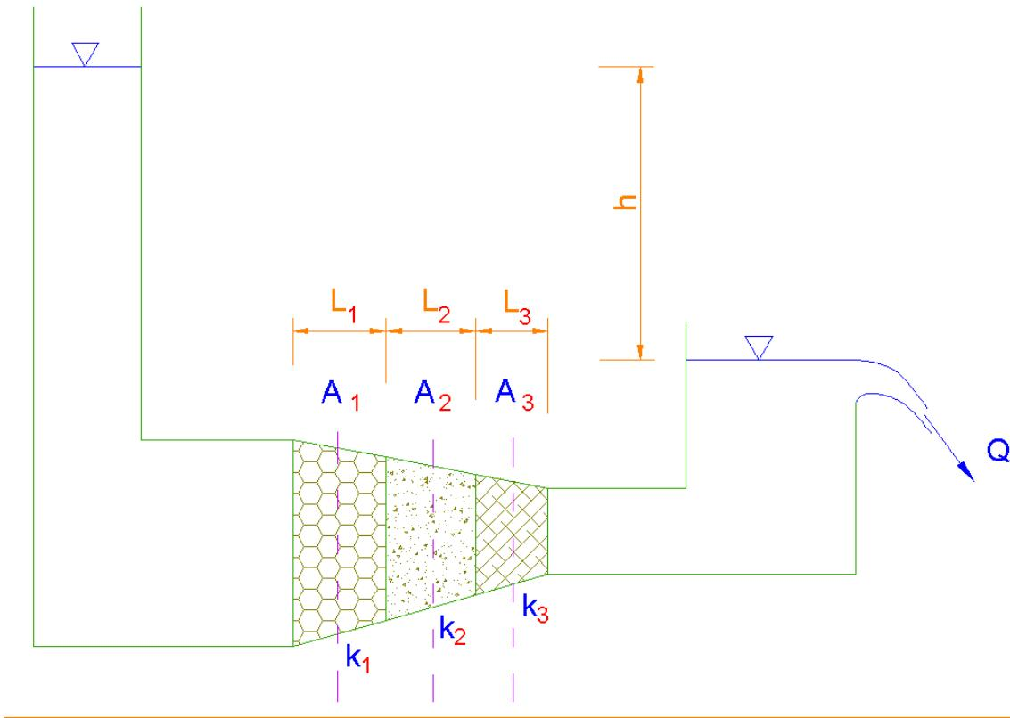
$$v_i = \frac{Q}{A_i} = -k_i \frac{\Delta H_i}{L_i} \Rightarrow \Delta H_i = \frac{Q \cdot L_i}{A_i \cdot k_i}$$
