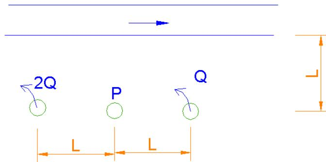
$$k \left( \frac{H^2 - h_Q^2}{2} \right) = \frac{Q}{2\pi} \ln \frac{R}{r_o} + \frac{2Q}{2\pi} \ln \frac{R}{2L} - \frac{Q}{2\pi} \ln \frac{R}{2L}$$
