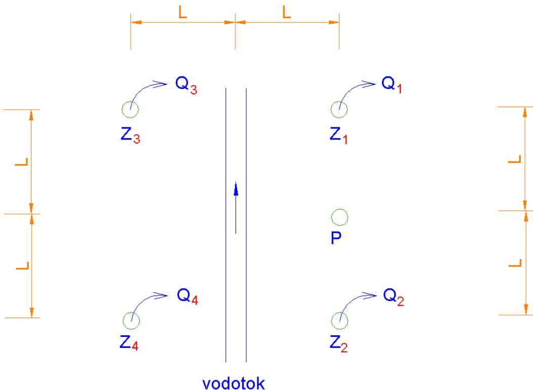
$$\Delta\Phi_p = \frac{Q_1}{2\pi} \ln \frac{R}{L} + \frac{Q_2}{2\pi} \ln \frac{R}{L} - \frac{Q_1}{2\pi} \ln \frac{R}{\sqrt{5}L^2} - \frac{Q_2}{2\pi} \ln \frac{R}{\sqrt{5}L^2}$$
