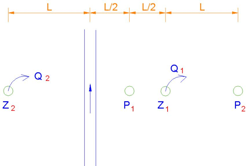
$$s_{P1} = \frac{Q_1}{2\pi k M} \cdot \ln \frac{R}{50} - \frac{Q_1}{2\pi k M} \cdot \ln \frac{R}{150} = \frac{Q_1}{2\pi k M} \cdot \ln \frac{\frac{R}{50}}{\frac{R}{150}} = 0,35 \text{ m}$$
